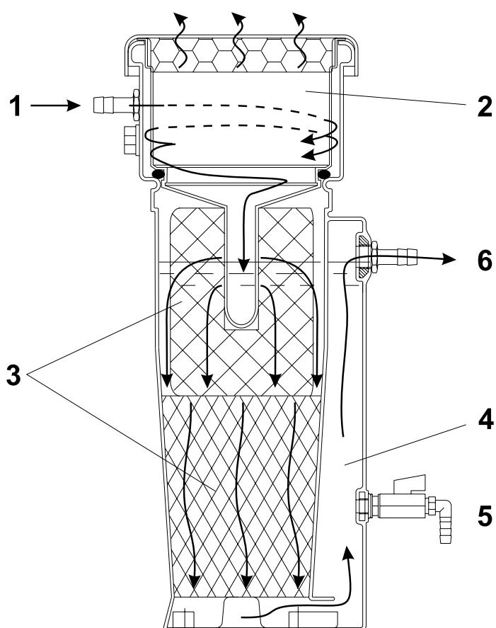
The oil-contaminated condensate can be fed under pressure to the QWIK-PURE unit (1).
