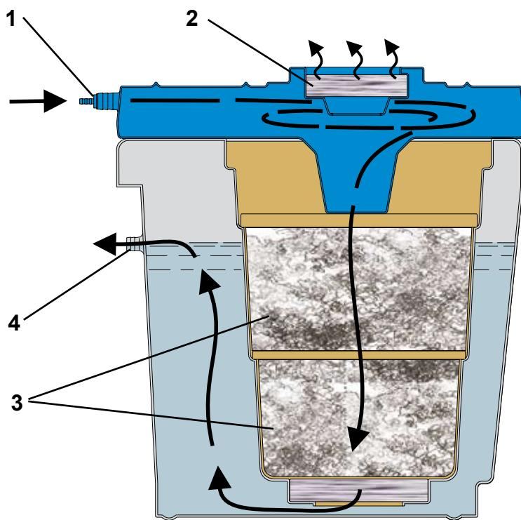
The oil-contaminated condensate can be discharged under pressure into the QWIK-PURE oil-water separator (maximum system pressure 16 bar).
